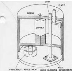
FIGURE 2. Sectional view of the tank circuit showing details of assembly
