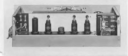
FIGURE 3. Rear view of the power-level indicator with dust cover removed. Note that all tubes are easily accessible from the rear
