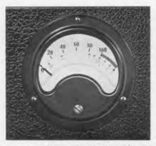
FIGURE 2. Photograph of the indicating meter. The main scale is black on a yellow background. The decibel scale is red. Two lamps behind the panel illuminate the scale
